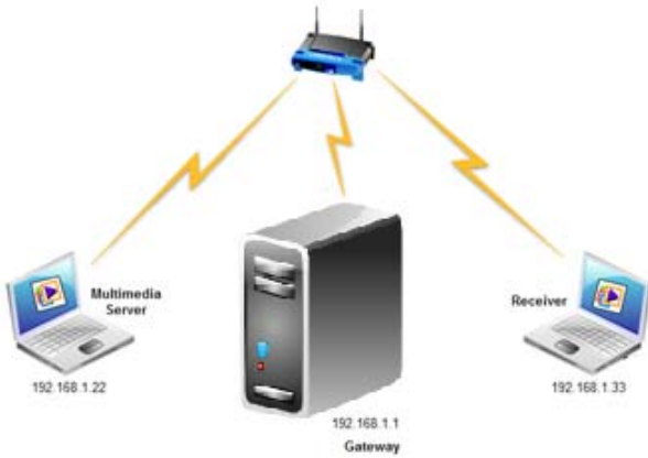
Figure 2. High Level Diagram of the Testbed Setup
