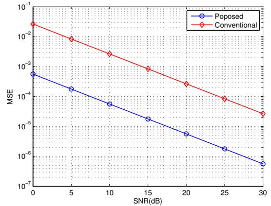
Fig. 1. Comparison of the Channel estimate MSE between the proposed preamble sequences and the equal powered trainings,  $N_t = 2$
