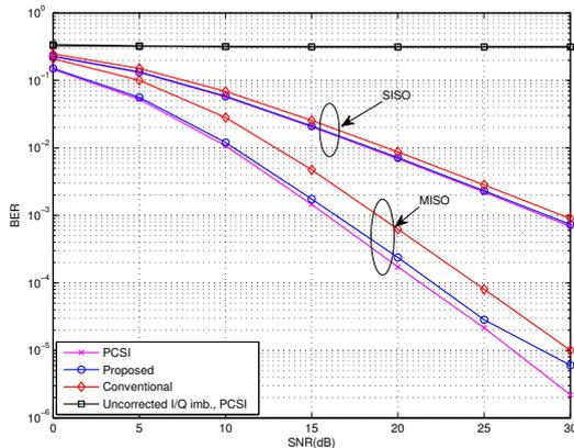
Fig. 2. BER versus SNR results for 64QAM constellation, phase imbalance of  $2^\circ$ , amplitude imbalance of 1dB and  $L = 4$
