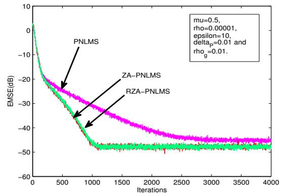
Fig. 2. The EMSE versus number of iterations for the standard PNLMS (pink), the RZA-PNLMS (green) and the ZA-PNLMS (red) algorithms.
