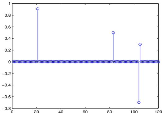
Fig. 1. Impulse response of the sparse system
