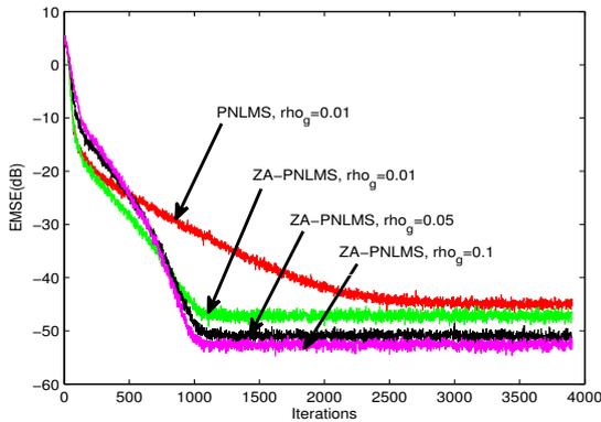
Fig. 3. The effect of  $\rho_g$  on the steady state EMSE of the ZA-PNLMS algorithm.
