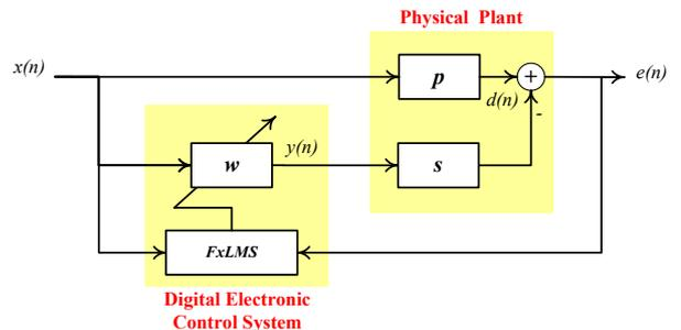
Figure 1: Functional block diagram of FxLMS-based ANC
