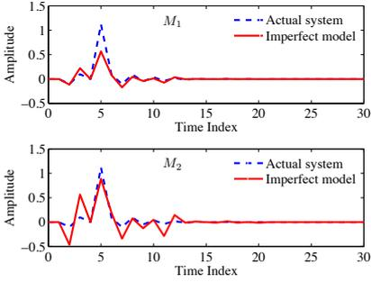
Figure 3: Impulse responses of secondary path models
