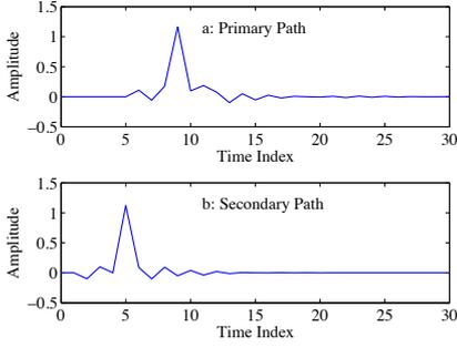
Figure 2: Impulse responses of primary and secondary paths in computer simulation
