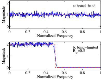
Figure 4: Power spectrum of two reference signals generated by computer ( $\sigma_x^2 = 1$ )
