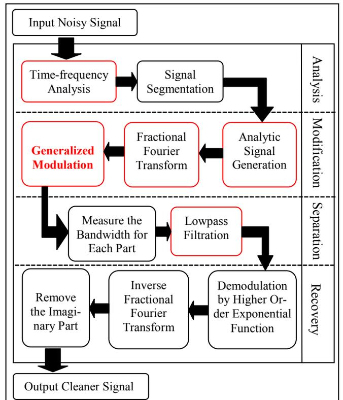
Fig. 1 Flowchart of the proposed noise-removing algorithm.
