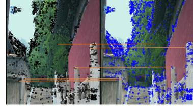
Fig. 2 Extracted feature points and the matched point pairs between the left view and right view of a stereo image.
