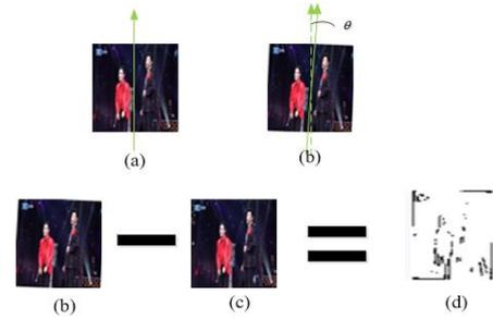
Fig. 5 Rotation detecting method. (a) original left image. (b) left image rotated by  $\theta$ . (c) original right image. (d) the difference between the rotated left image and the original right image
