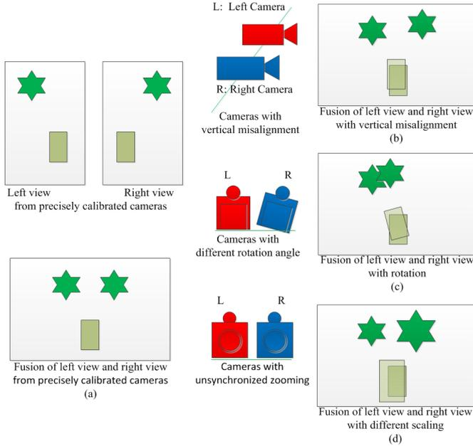
Fig. 1 Geometrical camera distortions [10].
