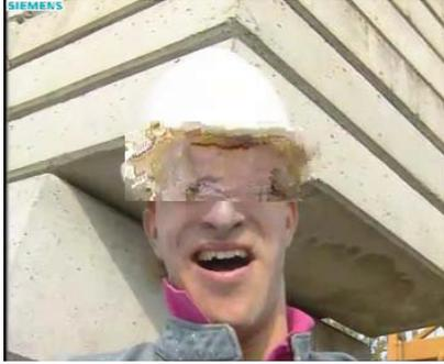
Fig. 8. The scrambled frame by modifying the  $MVD$  in  $16 \times 16$ ,  $16 \times 8$  and  $8 \times 16$  partitions. The average PSNR of privacy region is 16.23 dB.
