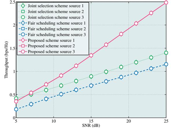
Fig. 3. Average per-source throughput versus SNR of different schemes with i.i.d. configuration.
