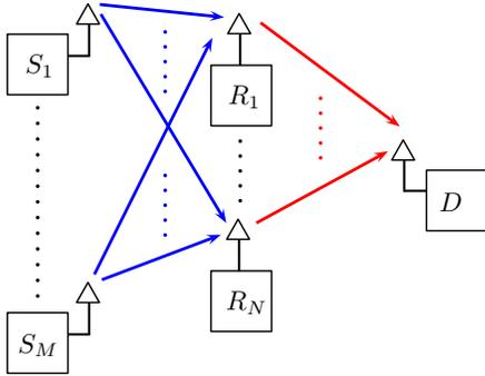
Fig. 1. A cooperative wireless network where  $M$  source nodes communicate to a common destination node with the aid from  $N$  relay nodes.
