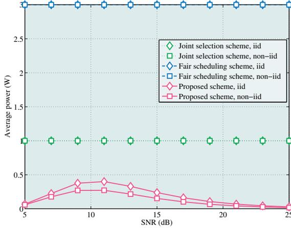
Fig. 2. Average relay power consumption versus SNR for different schemes.
