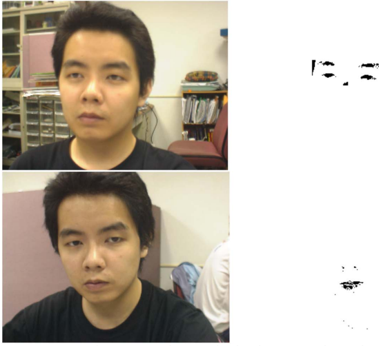
Fig.5: Extraction results for the eyes and mouth
