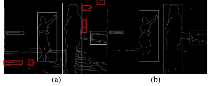
Fig. 8 Correspondent object selection. (a) Objects selected in depth image; (b) I_{AND} image.
