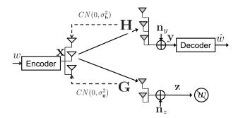
Fig. 1. Fast Rayleigh fading MIMOME wiretap channel with statistical CSIT.
