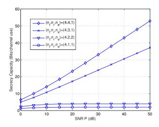
Fig. 2. Subject to total power constraints, the secrecy capacities versus SNRs with different number of antennas and  $\sigma_h^2/\sigma_g^2 = 4$ .
