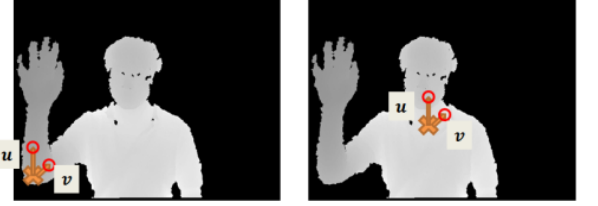
Fig. 8. Properly selected split parameter \theta = \{\mathbf{u}, \mathbf{v}\} with different f_\theta value can be used to differentiate the class of the patch sample.
