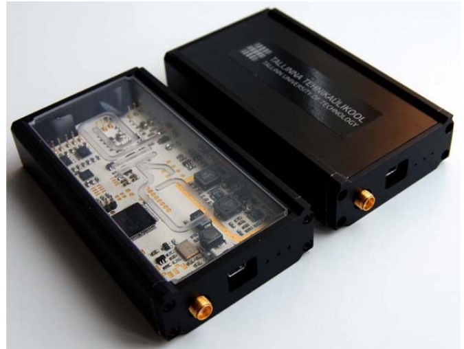
Fig. 3 Photography of the first version of the DSP-based signal processing module prototype.
