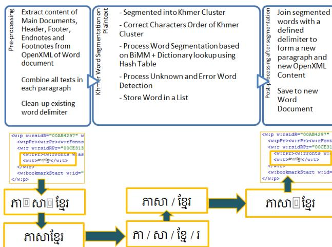
Fig. 3 Process Flow of Khmer Word Segmentation for Word Document
