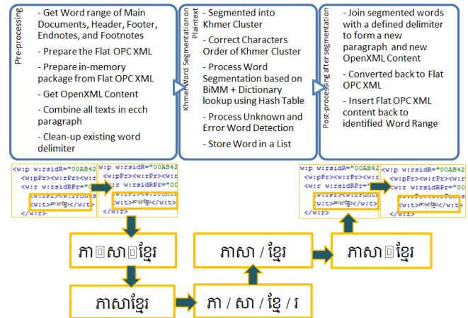
Fig. 4 Process Flow of Khmer Word Segmentation for Current Opened Word Document
