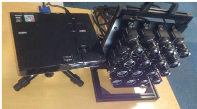
Fig. 3. Our camera array and projector system
