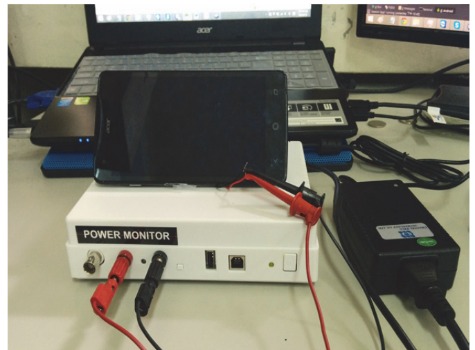
Fig. 7. The Acer Liquid S1 and Monsoon’s power monitor used in our experiments.
