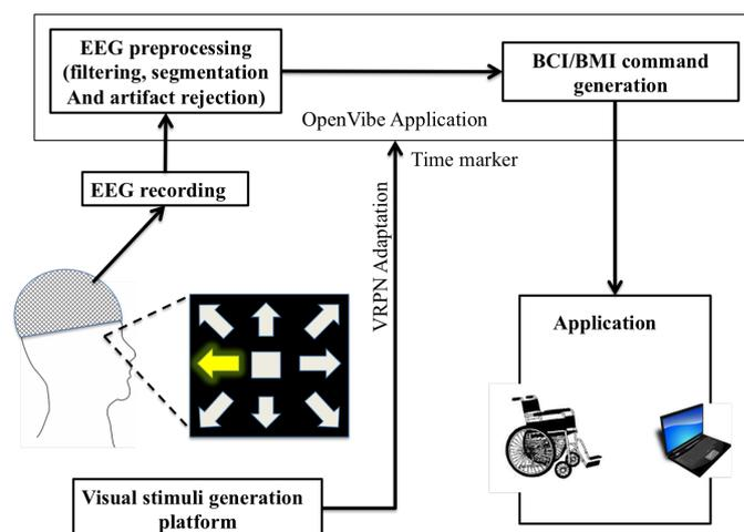
Fig. 1. Schematic diagram of the spatial visual BCI application. EEG signals are processed and classified by OpenVibe [7] software processing stages in synchrony with presented visual stimuli to generate interactive commands.
