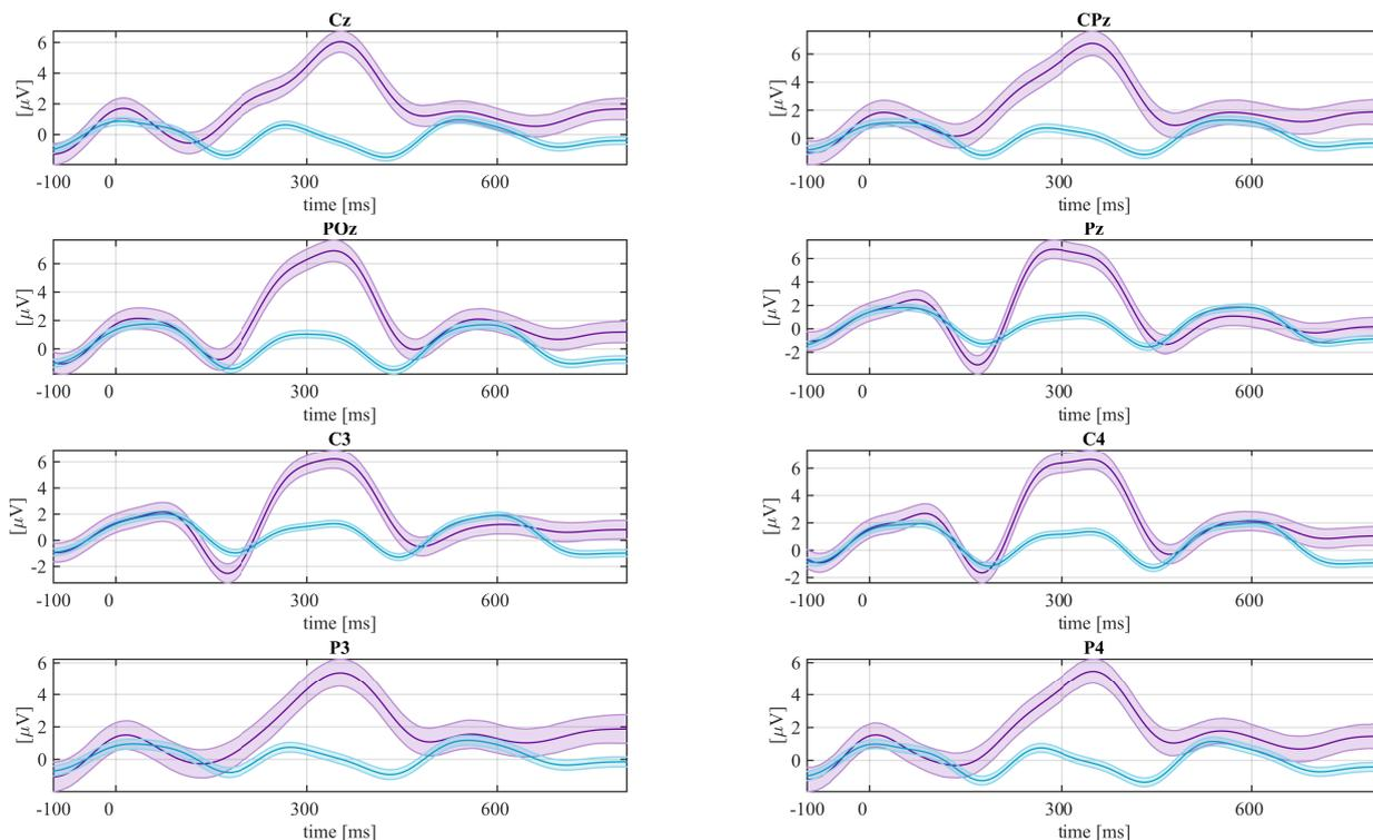
Fig. 3. The grand mean average ERP brain responses of the protocol one ( $ISI = 200$  ms) with purple and blue middle lines depicting targets and non-targets, respectively. Standard error intervals are visualized also around the mean traces.
