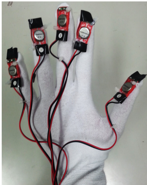
Fig. 2. The fingertip-sense glove used in the experiments. Five vibrotactile transducers are attached at fingertips.
