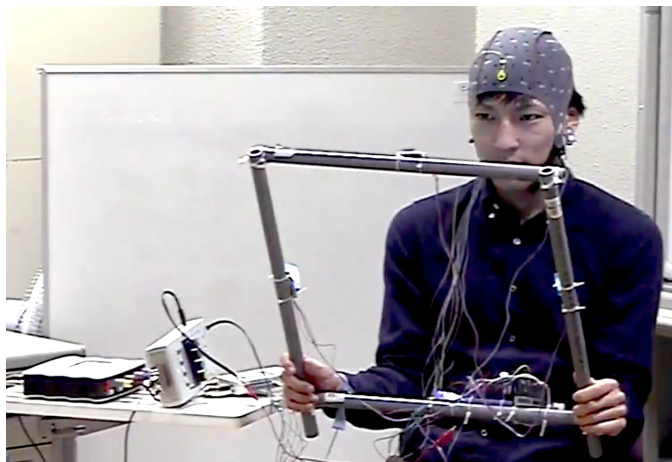
Fig. 1. A user holding a frame with four LEDs attached to each edge. The user is wearing the EEG cap and g.USBamp amplifier on the left together with a trigger capturing box g.TRIGbox, all by g.tec medical instruments GmbH, Austria, are also presented. The photograph is reproduced with the user's consent.
