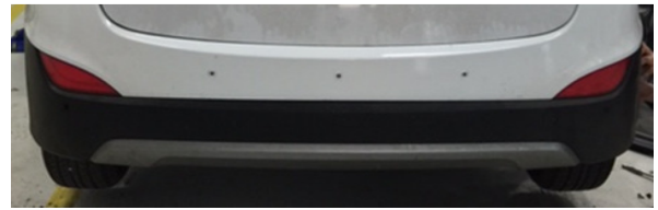
Fig. 1 the equipped multiple microphones in the rear bumper of test vehicle.
