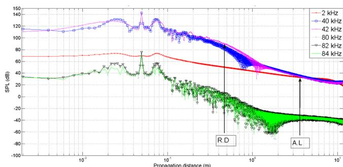
Fig. 6 On-axis sound pressure level of the 50 transducers loudspeaker.
