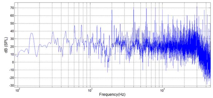
Fig. 3 FFT of the 195 transducers loudspeaker simulated.
