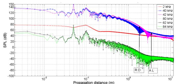
Fig. 8 Axial sound pressure level of the 195 transducers loudspeaker.
