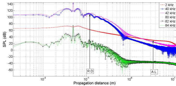
Fig. 5 On-axis sound pressure level of the 13 transducers loudspeaker
