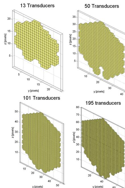
Fig. 4 Loudspeakers simulated of 13, 50, 101 and 195 transducers.
