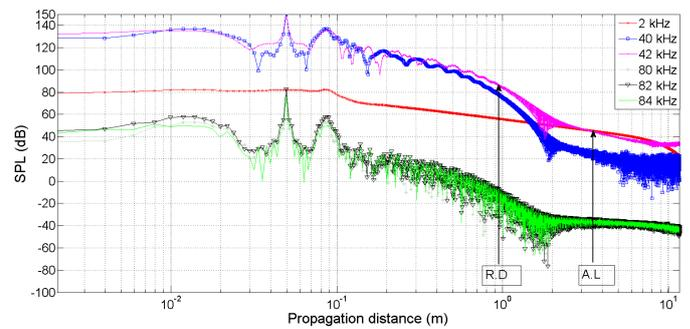
Fig. 7 Axial sound pressure level of the 101 transducers loudspeaker.
