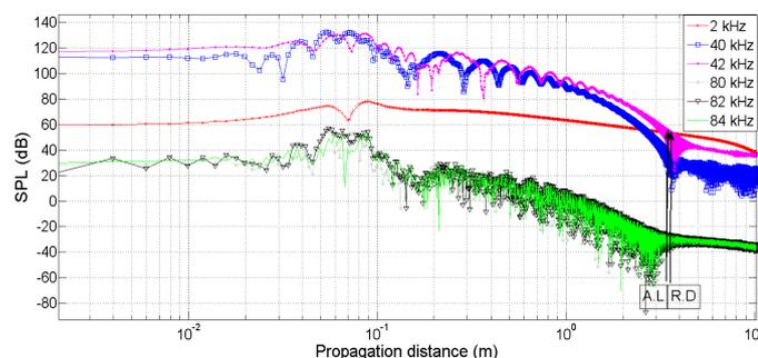
Fig. 10 On-axis sound pressure level of the 397 transducers loudspeaker.
