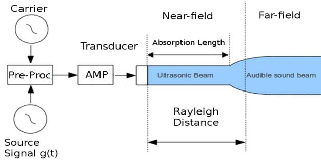
Fig. 1 Diagram of a parametric loudspeaker and its acoustic field.
