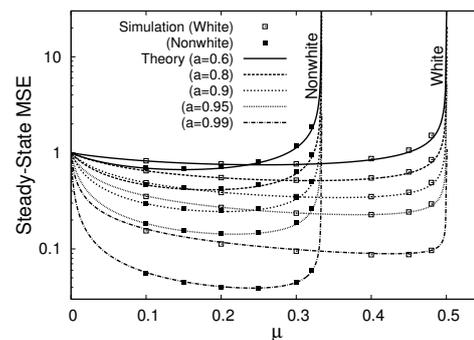
Fig. 3. Relationship between step size  $\mu$  and steady-state MSE obtained theoretically and by simulation.
