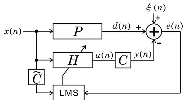
Fig. 1. Block diagram of the ANC system.
