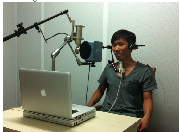
Fig. 1 Data collection system showing ultrasound and EMA devices
