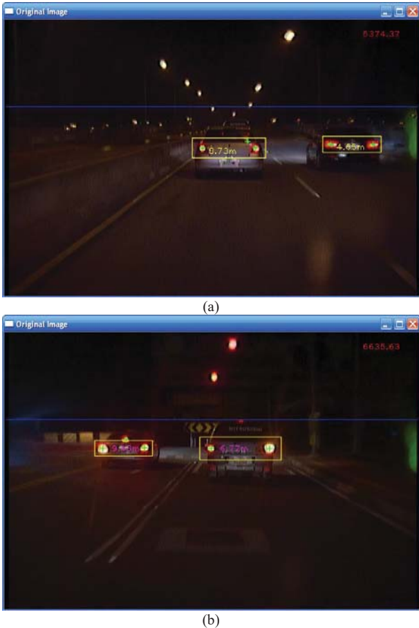
Fig. 8. The experimental results of (a) two vehicles run in parallel. (b) The size of a rear light pair is different when the turn signal is on.
