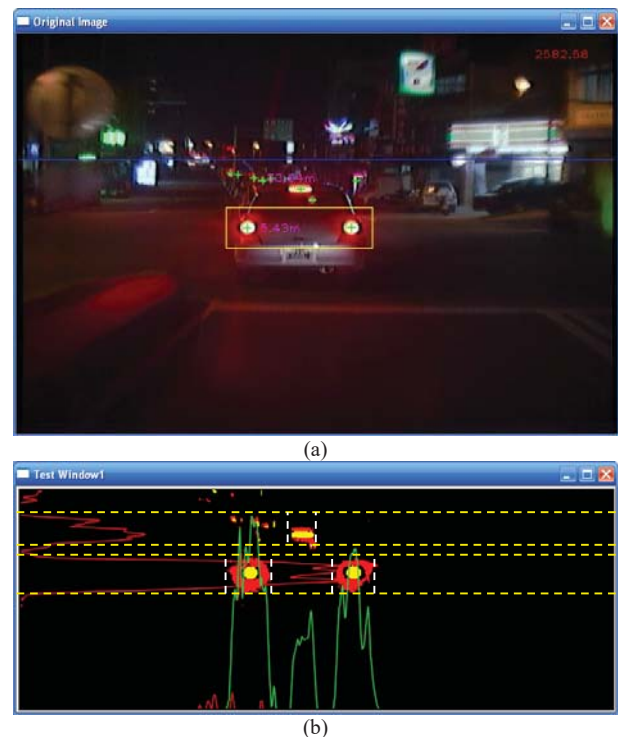
Fig. 4. The rear light segmentation. (a) The original image. (b) After horizontal and vertical projections, the extracted rear lights are enclosed by bounding boxes.
